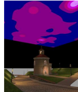
Figure 5. Virtual model of Scenarios – realistic rendering (left) and luminance distribution calculation (middle) and upward light emission view (right)
